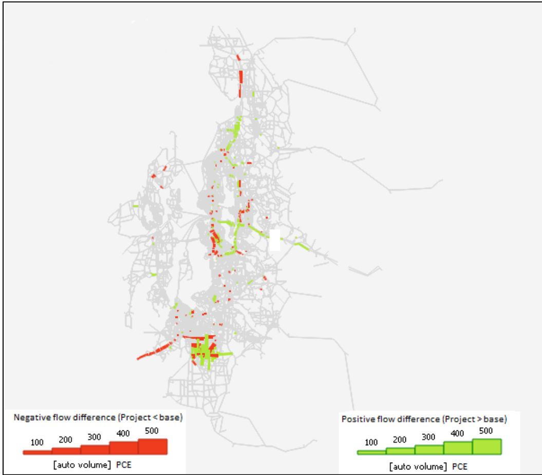
Figure 7-54 Flow Differences in the PSRC Network at 1.E-5 Convergence
